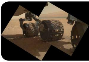
The view of the three left wheels combines two images taken by the rover's Mars Hand Lens Imager.
