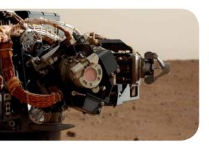
The Mars Hand Lens Imager (MAHLI) is one of the tools on a turret at the end of the rover's robotic arm.
