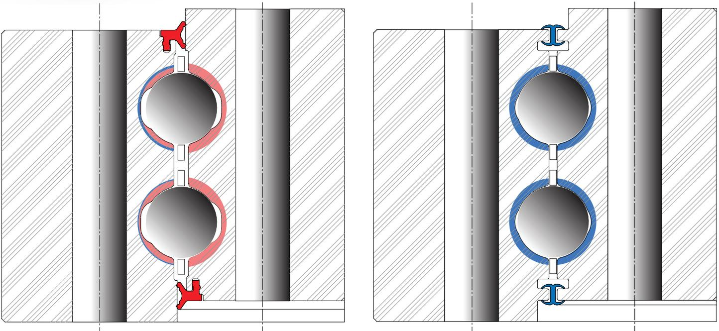
Recommended case depth shown in blue; actual case depth of failed bearing (left) shown in red. The failed bearing features rubber seals, which are replaced with an 'H' seal cross-section profile in the bearing upgrade (right).
