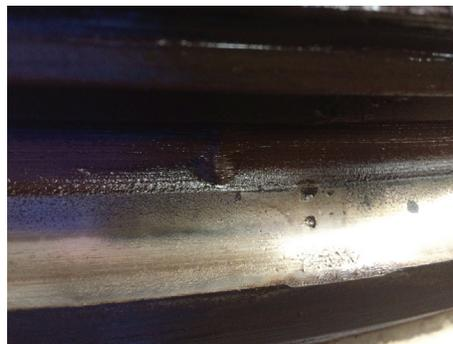
Denting and corrosion
