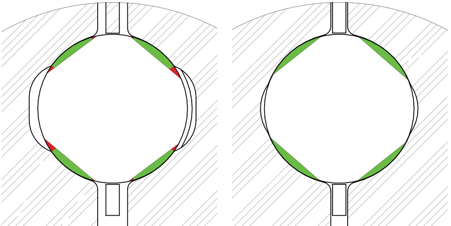
The contact pattern of an OEM pitch bearing (left) vs the bearing upgrade (right). Contact truncation indicated in red.
