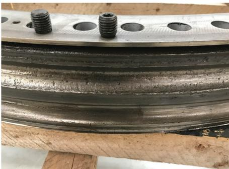
Core crushing and cold working
